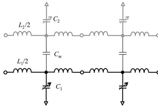
Fig. 1. Two adjacent cells of a coupled NTL.
