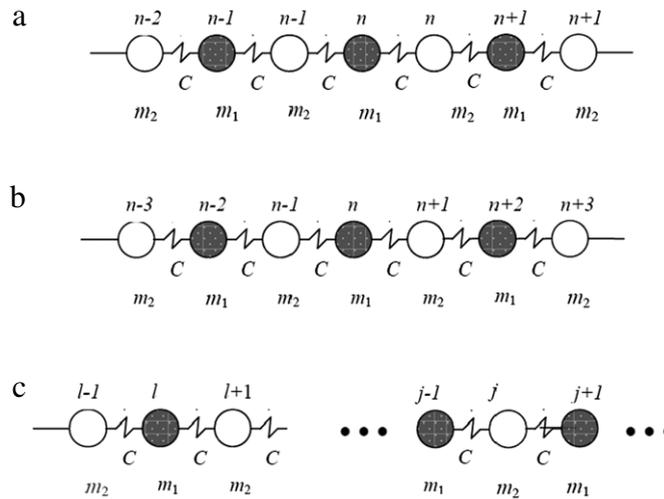
**Fig. 1.** Numbering of the masses in the lattice for different models: (a) pair or double numbering, (b) consecutive numbering, (c) numbering suitable even for non-neighboring masses.
