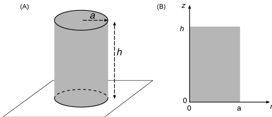
Fig. 1. Capped cylinder electrode (A); geometry for simulation (B).
