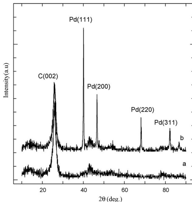
Fig. 1. XRD patterns for MWCNTs (a) and Pd/MWCNTs (b).
