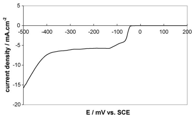
Fig. 2. Voltammogram in 1 M  $\text{HNO}_3$ ,  $[\text{Te}^{\text{IV}}] = 2 \times 10^{-2}$  M,  $[\text{Bi}]/[\text{Te}] = 1$ , working electrode: stainless steel, surface area = 1.24  $\text{cm}^2$ , counter electrode: platinum disc, scan rate = 60  $\text{mV min}^{-1}$ .
