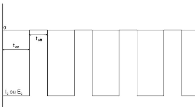
Fig. 1. Theoretical diagram of the pulse plating electrodeposition process.
