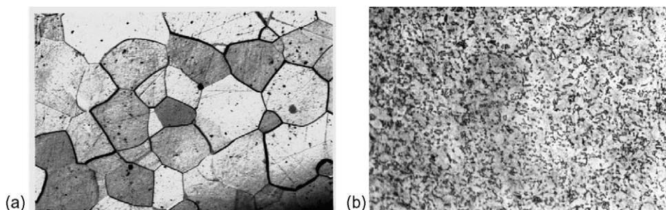
Fig. 1. Photomicrographs of the Ti (a) and Ti6Al4V alloy (b) surfaces etched with a Kroll reagent (200 $\times$ ).
