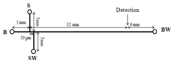
Fig. 1. Dimensions and layout of the glass/PDMS microchip used in this work: S, sample reservoir; B, buffer reservoir; SW, sample waste reservoir; and BW, buffer waste reservoir.
