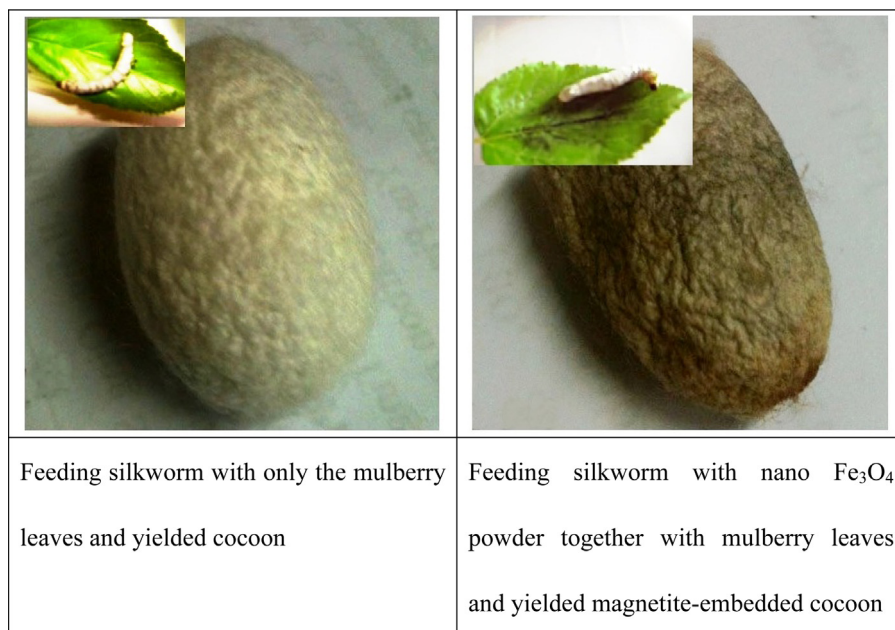
Fig. 1. The macroscopic images of the normal feeding of silkworm with only mulberry leaves and the yielded cocoon (left) and the feeding of nano \text{Fe}_3\text{O}_4 powders together with the mulberry leaves and the yielded magnetite-embedded cocoon (right).
