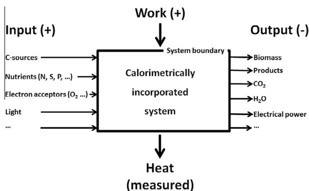
**Fig. 1.** Calorimeter as an open system exchanging energy and matter with the environment. The calorimeter can incorporate parts of ecosystems, bioreactors or simple samples with living matter. The system can be in steady state or in a transient. It has to be adapted to the specific experimental conditions. Convective heat flows due to exchange of matter is not considered. The figure is derived from [9].
