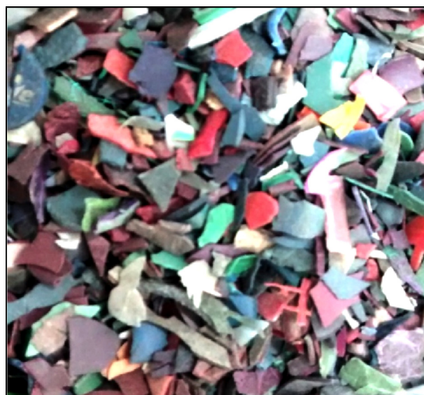
Fig. 1. Plastic waste sample (shredded and sieved).
