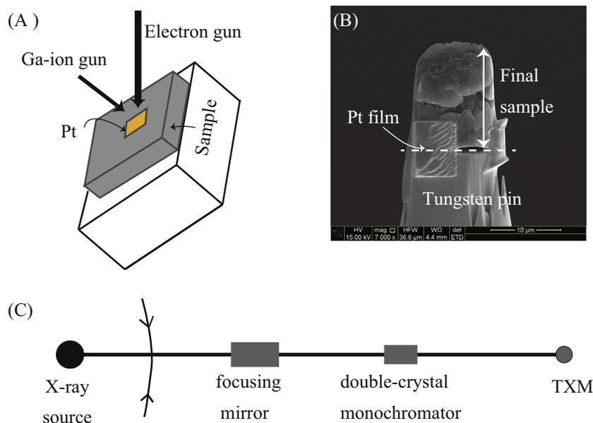
**Fig. 1.** (A) Schematic drawing of the milling procedure in a FIB dual-beam system. (B) Side-view of the final sample for Nano-TXM investigation. (C) Optical layout of beamline BL01B at the NSRRC.
