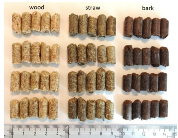
Fig. 1. Dimensions of selected biomass pellets: measurements of diameter and length were done by a vernier caliper.
