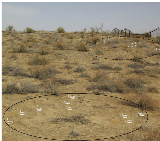
Fig. 1. Experimental plots covered by moss-dominated crusts (surrounded by solid line) and mixed crusts (surrounded by dashed line), with tubes for control (1) and for simulation of shallow (2) and deep (3) sand burial.
