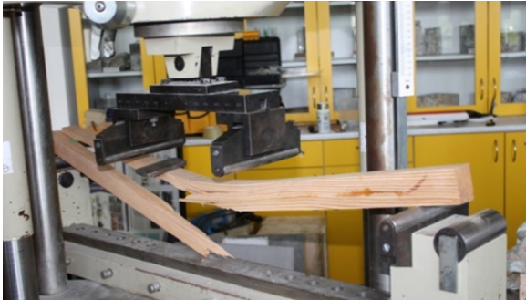
Figure 2 Implementation of the strength test on wooden samples.
