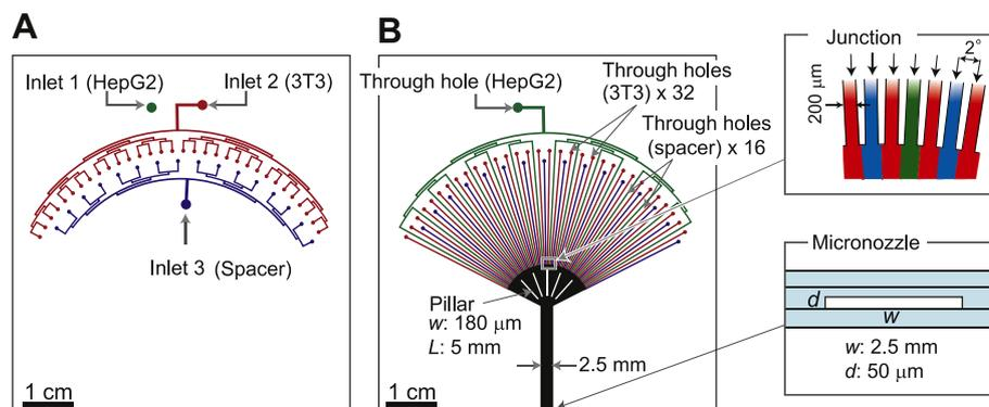
FIG. 2. Microchannel design for preparing stripe-patterned hydrogel sheets. This device was fabricated by layering 3 PDMS plates; a top (A), a middle layer (B), and a flat bottom layer.
