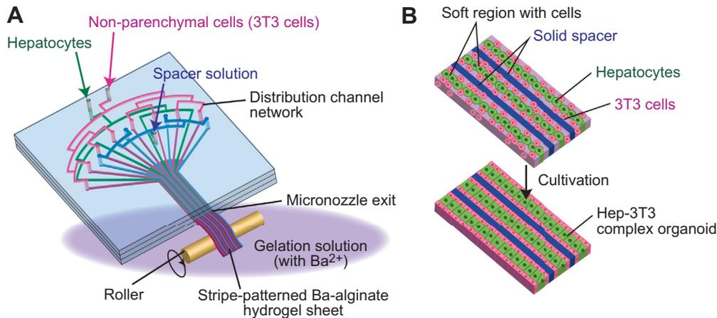
FIG. 1. Schematic showing the preparation procedure of the stripe-patterned heterogeneous hydrogel sheet (A) and formation of heterotypic micro-organoids in the soft/solid hydrogel sheet (B).
