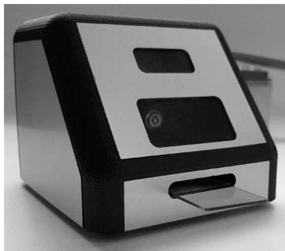
Fig. 1. Trumorph® system prototype. See the heating stage with the pressure mechanism.
