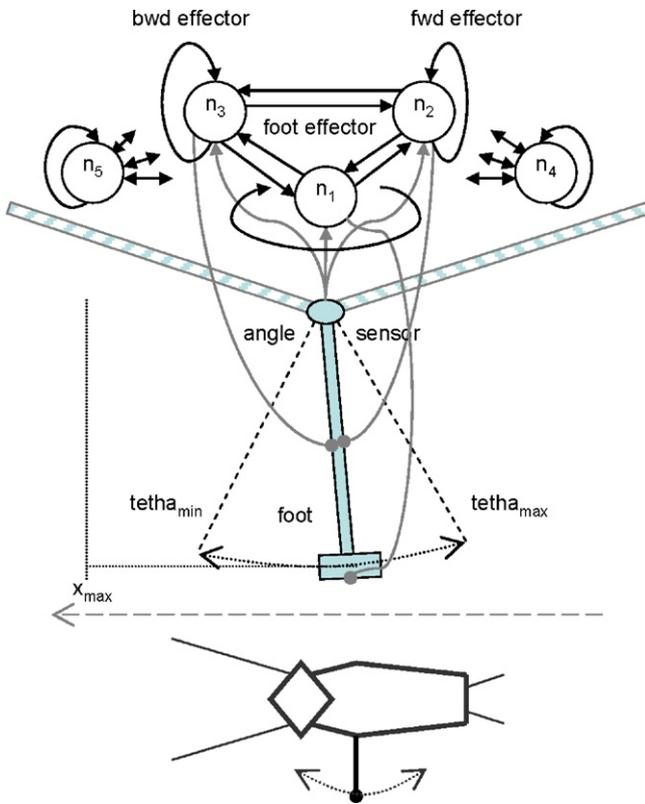
**Fig. 1.** (Top) Schematic representation of the agent's leg configuration for one-legged walking behaviour. Neurons are fully connected including self-connections. Three effectors controls the forward and backward force applied to the leg and the foot for walking. Effectors receive sensory stimuli of the leg angle during the ongoing task. (Bottom) The leg model of a simulated insect where the leg can swing about their single joint with the body (figure based on Beer (1995a)).
