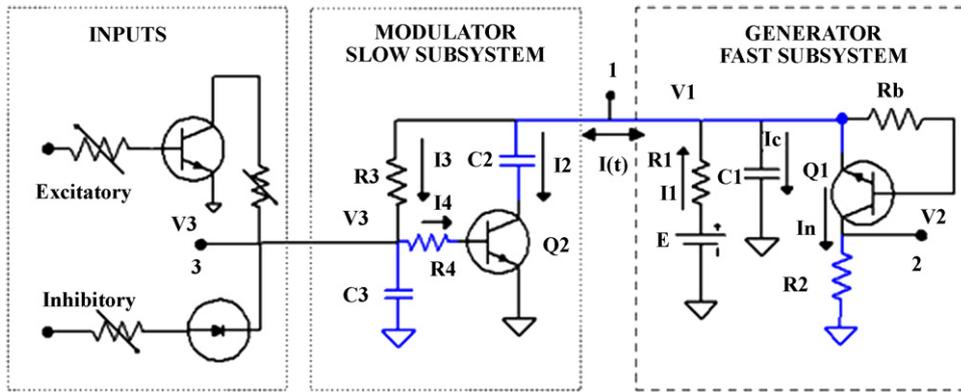
**Fig. 1.** The bursting and spiking analog circuit. The “frequency adaptation loop” includes C3, R4, Q2 base–collector junction, C2, Q1 emitter–collector junction and R2. Transistors Q1 (reverse-biased) and Q2 are 2N2222 type, battery  $E = 10\text{ V}$ , resistance value in  $\text{K}\Omega$  and capacitances in  $\mu\text{F}$ :  $R1 = 3.3$ ,  $R2 = 0.1$ ,  $R3 = 100$ ,  $R4 = 1$ ,  $Rb = 50$ ,  $C1 = 1$ ,  $C2 = 10$ ,  $C3 = 2$ .
