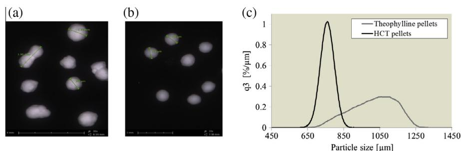
Fig. 1. Core material: (a) theophylline pellets, (b) HCT layered pellets (light microscopic pictures), (c) volume density distributions ( $q_3$  [%/ $\mu\text{m}$ ]) measured by the dynamic image analysis. (For interpretation of the references to color in this figure legend, the reader is referred to the web version of this article.)
