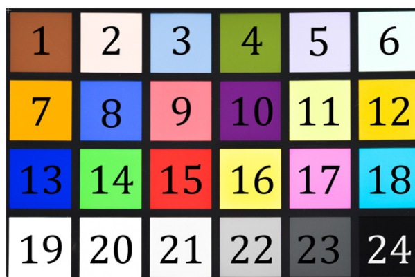
Fig. 1. The X-Rite color-chart used in the experiments. It provides a set of gray levels on the bottom row. Several colors, properly distributed in the color space, allow the evaluation of color fidelity of the acquisition system: the expected L*a*b* values are provided by the manufacturer.
