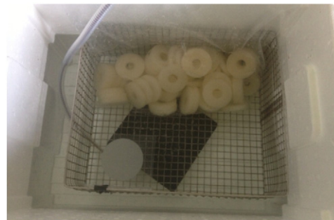
Fig. 1. Experimental set-up for the elution using megasonic sonication. The sponge filters, seen at the top of the figure have a doughnut shape when fully expanded and are enclosed in a plastic bag. The membrane is seen in a smaller bag on the bottom left of the figure. The megasonic transducer, seen as a black square, is placed at the bottom of the bath filled with water.
