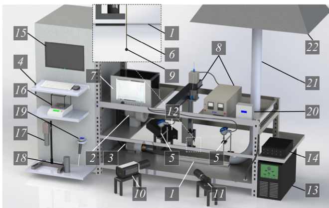
Fig. 1. Schematic of the experimental setup [23]: 1—hollow glass cylinder; 2—air fan; 3—heater; 4—remote control; 5—thermocouples; 6—tip (or low-inertia thermocouple); 7—recorder; 8—mini-robotic arm; 9—CWSP droplet; 10—high-speed video camera; 11—cross-correlation camera; 12—laser; 13—laser generator; 14—laser and cross-correlation camera synchronizer; 15—computer; 16—analytical balance; 17—homogenizer; 18—vessel with CWSP; 19—electronic dispenser; 20—gas analyzer; 21—ductwork; 22—ventilation.
