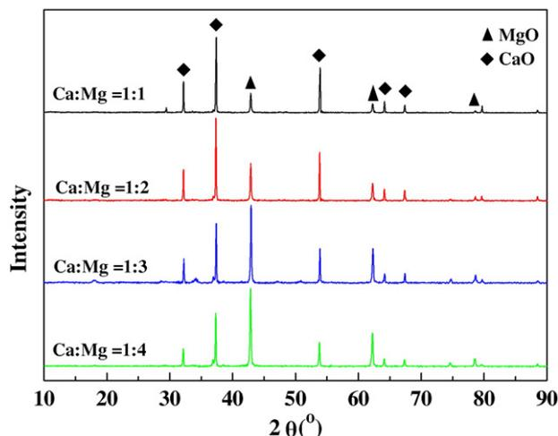
Fig. 1. XRD characterize patterns of different molar ratio of Ca/Mg catalysts.
