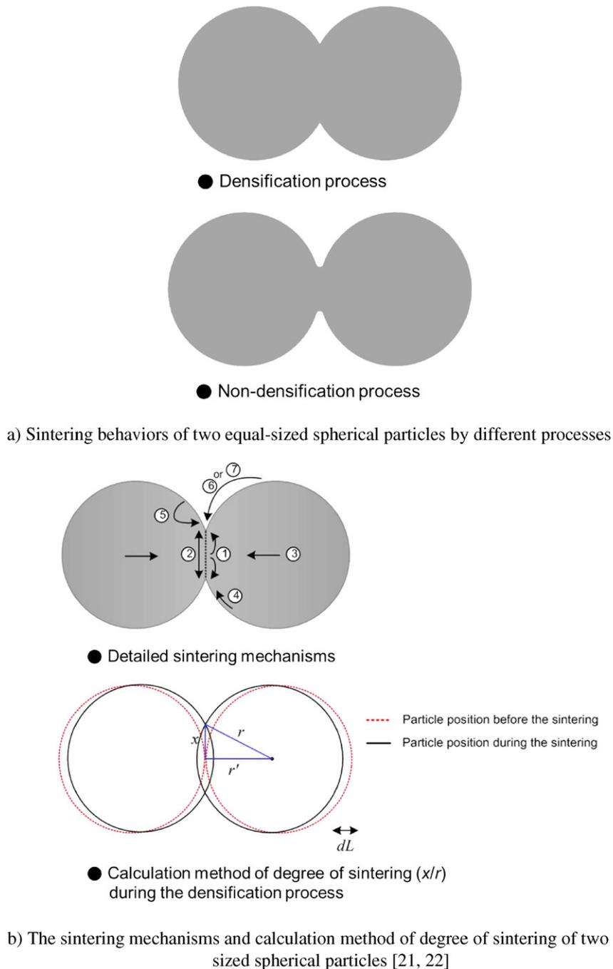
Fig. 1. Theoretical example for the particle sintering.
