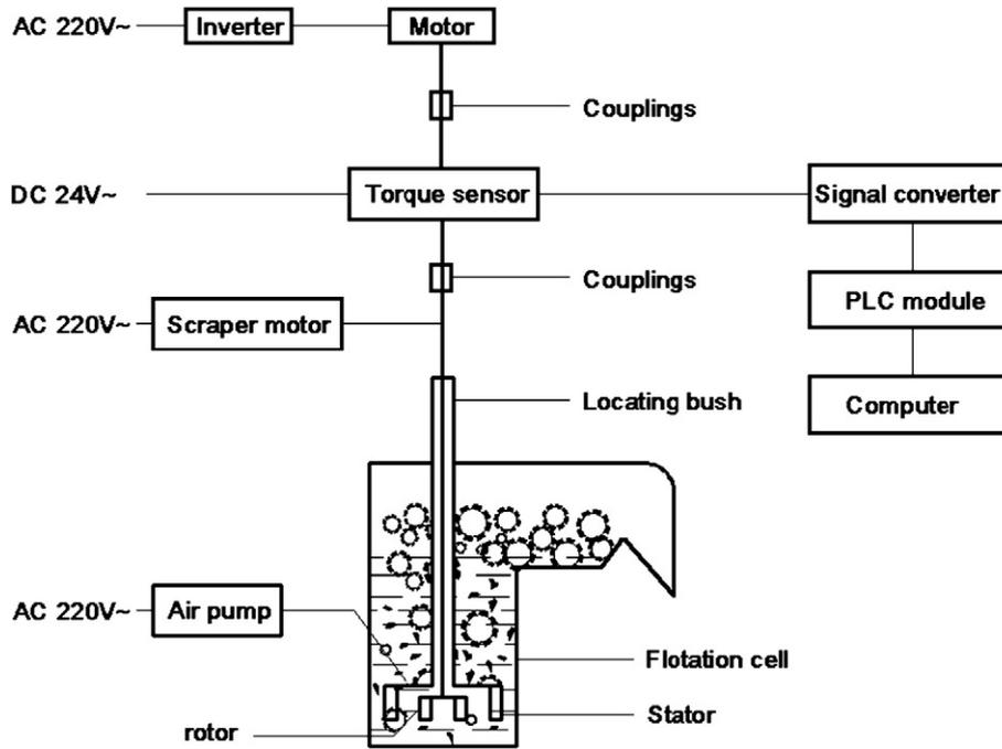
Fig. 1. Connected chart of flotation energy input measurement system.
