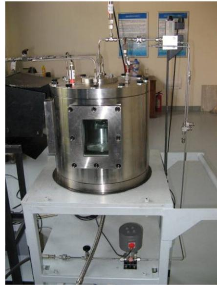
Fig. 2. The high-pressure spray visualization chamber.
