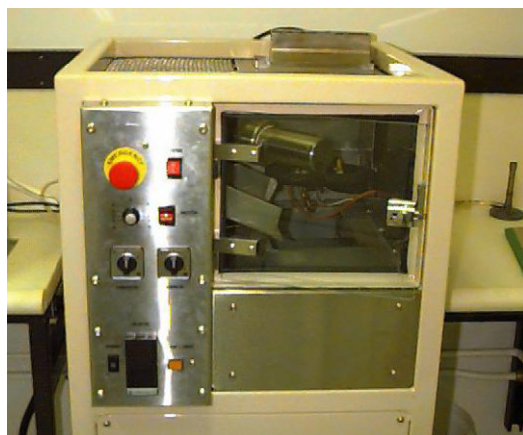
Fig. 1. Gas Fired Reactor (LHS, stainless steel bomb mounted horizontally) and an example of a time–temperature profile (not indicative of actual profiles used in the present work – shows heat-up and cool down rates and temperature stability).
