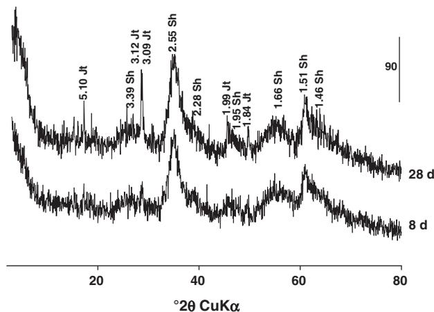
Fig. 1. X-ray diffractograms of precipitates formed in the absence of Pb-nitrate. Schwertmannite is the dominant phase in both 8 day and 28 day Pb-free samples. Peaks due to schwertmannite and a jarosite phase are identified as Sh and Jt, respectively. Numerical values are  $d$  spacings in Ångstrom units. The vertical bar indicates the scale of relative counts.
