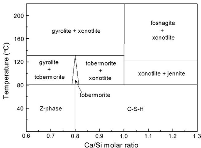
Fig. 1. Schematic stability diagram showing the relative stability of part of the hydrated calcium silicates (data are collected from Shaw et al., 2000, and Hong et al., 2004).
