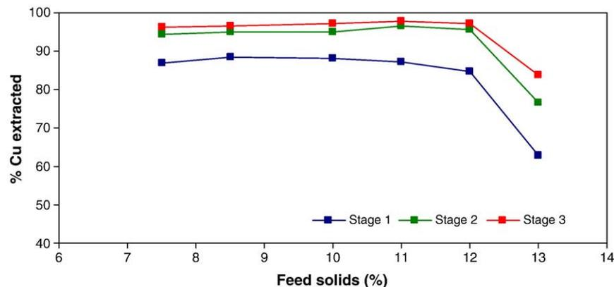
**Fig. 1.** The effect of feed solids concentration on Cu recoveries while operating at 70 °C.
