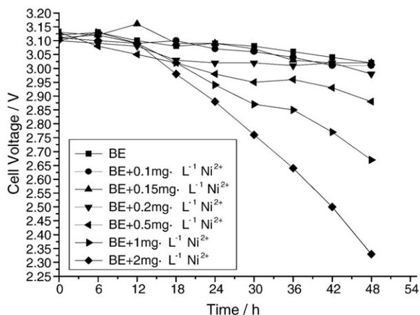
Fig. 2. The trend line of CV for 48 h zinc electrowinning.
