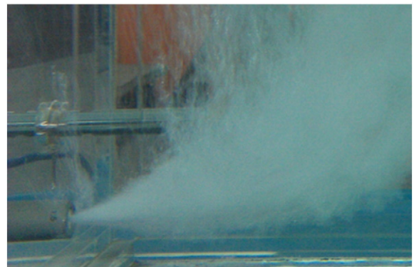
Fig. 3. Fine bubbles in water produced by KYZ-B sparger.
