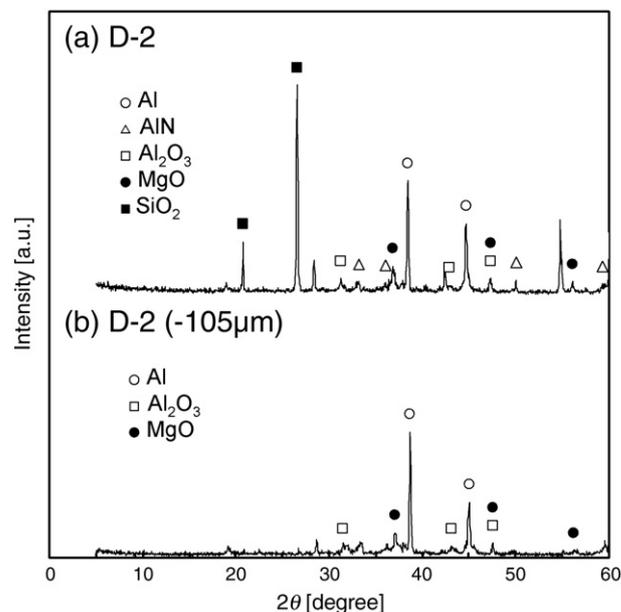
Fig. 2. XRD pattern of (a) aluminum dross D-2 and (b) D-2 ( $-105\ \mu\text{m}$ ) after classification.
