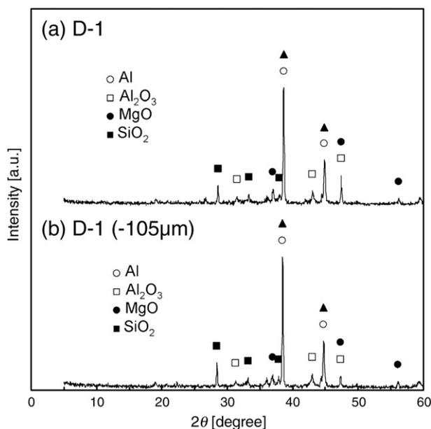
Fig. 1. XRD pattern of (a) aluminum dross D-1 and (b) D-1 ( $-105\ \mu\text{m}$ ) after classification.
