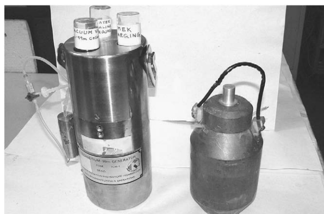
Fig. 2. A prototype technetium-99m generator using the solid–liquid extraction technique.
