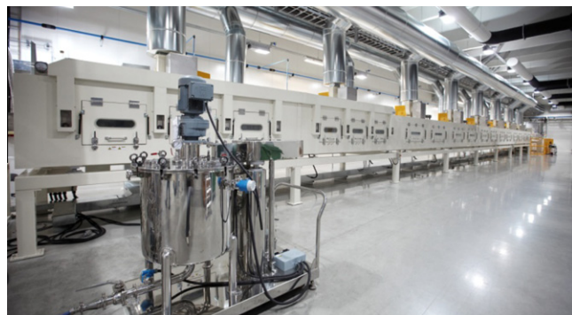
FIGURE 3. Overview of one of LFP electrode coating lines in European Batteries plant at Varkaus, Finland. The annual capacity of the plant is 100 MWh [9].
