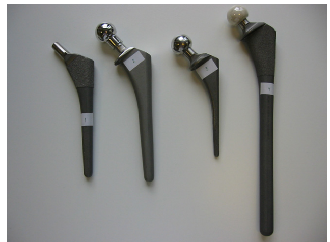
Fig. 2. Four different types of hip prostheses listed from 1 to 4. These prostheses are commonly used for patients undergoing hip surgery. Hip prosthesis no. 2 is Co–Cr–Mo alloy, the other three are Ti alloys. The head/junction is made of either stainless steel or ceramic materials. The ceramic head is used for hip prostheses no. 1 and no. 4.
