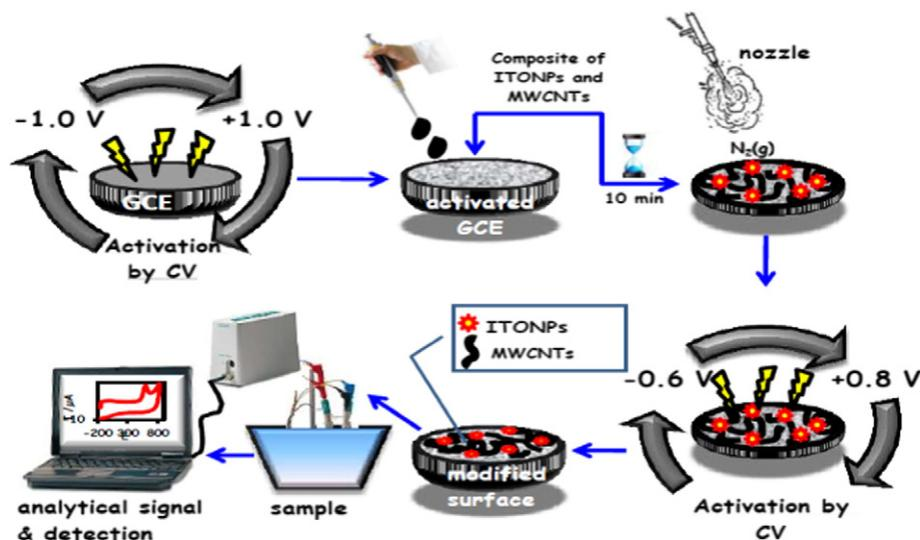
Scheme 1. An illustration of the preparation of the proposed electrode.
