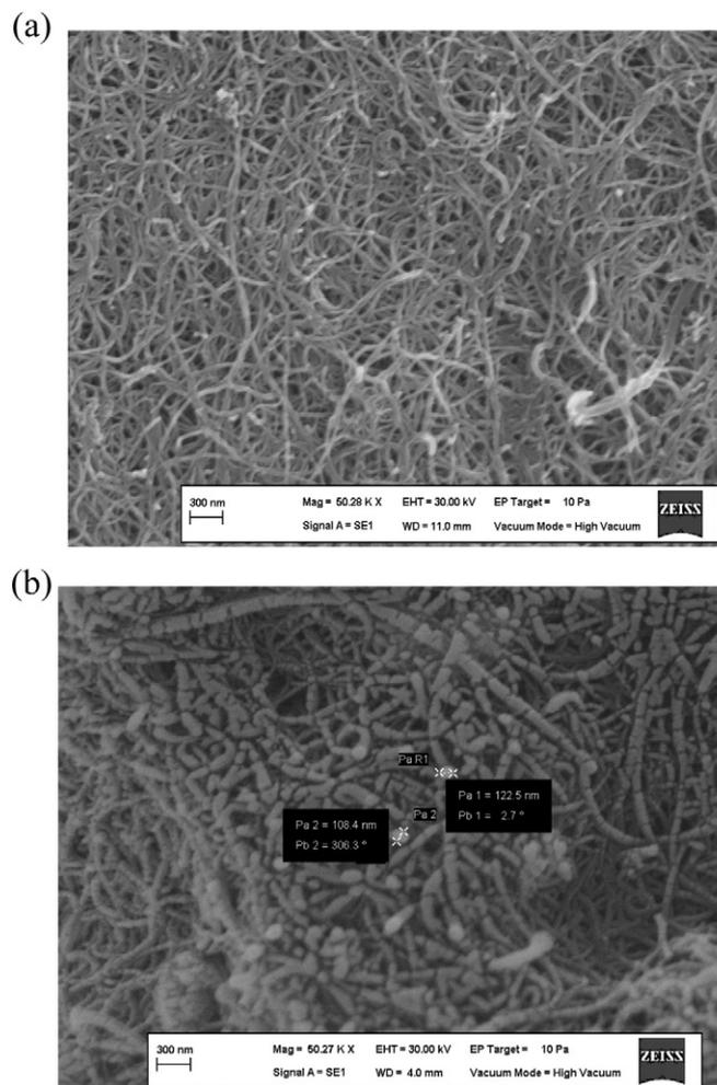
Fig. 1. SEM images of MWCNTs/GCE (a) and ITONPs/MWCNTs/GCE (b).
