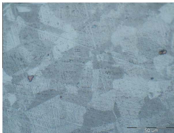
Fig. 1. Microstructure of Alloy 800 with an average grain size 20 \mu\text{m} after etching with Marble's agent (10 g copper(II) sulfate, 50 mL concentrated HCl and 50 mL water) for 15 s.
