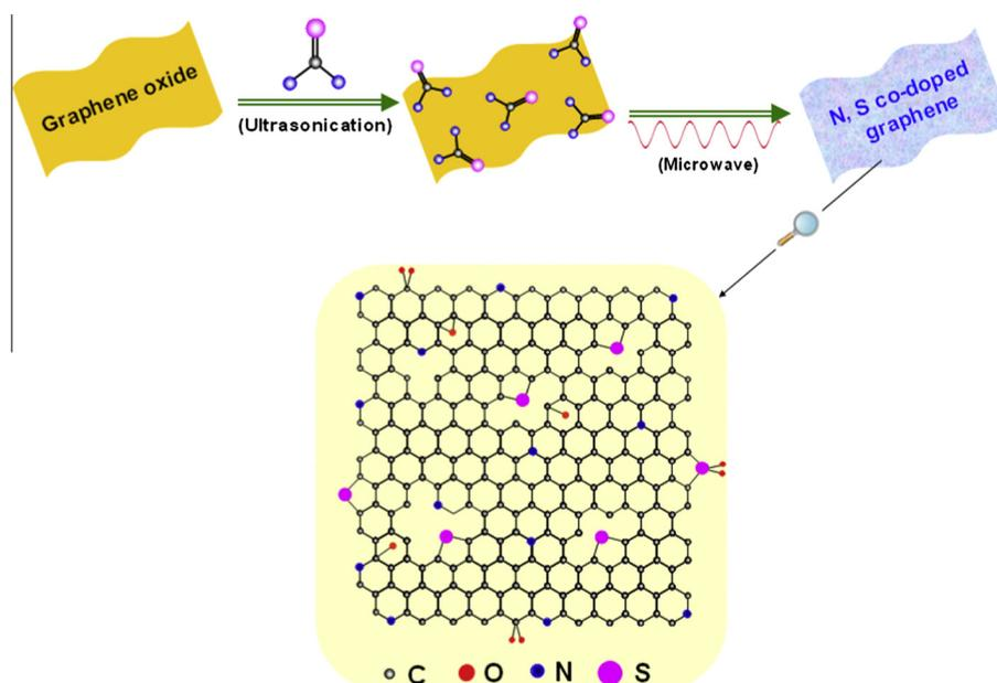
Fig. 1. Schematic illustration of the synthesis process of NS-G.
