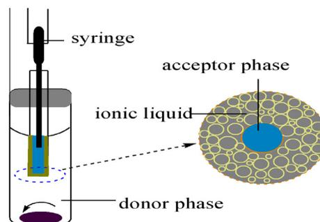
Fig. 2. The schematic plot of liquid–liquid–liquid phase microextraction (LLLME) based on hollow fiber supported ionic liquid membrane.
