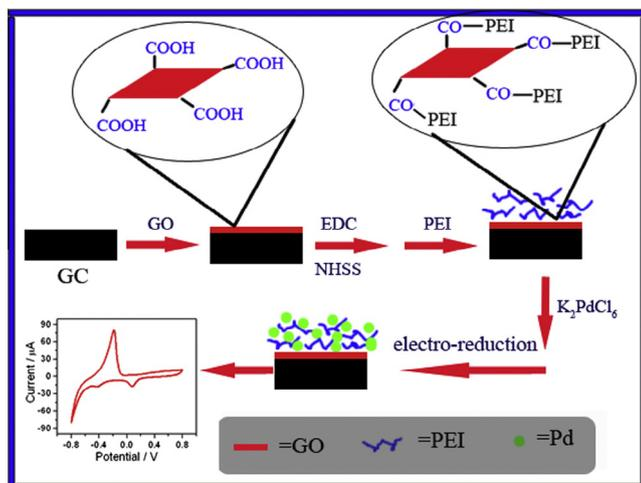
Fig. 1. Schematic representation for the fabrication processes of Pd-PEI/GO/GC electrode.
