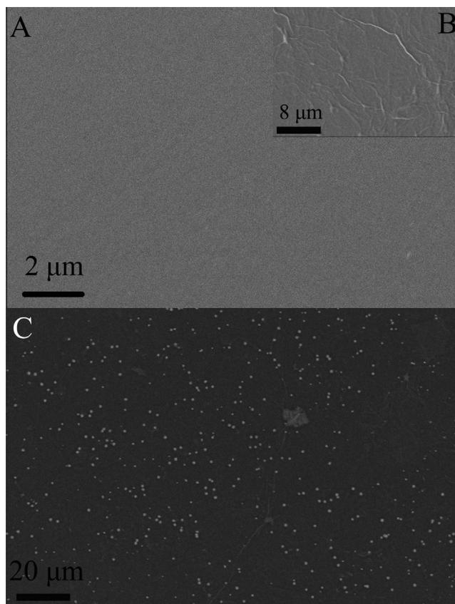
Fig. 2. SEM images of GC (A), GO/GC (B), and Pd-PEI/GO/GC (C) electrodes.
