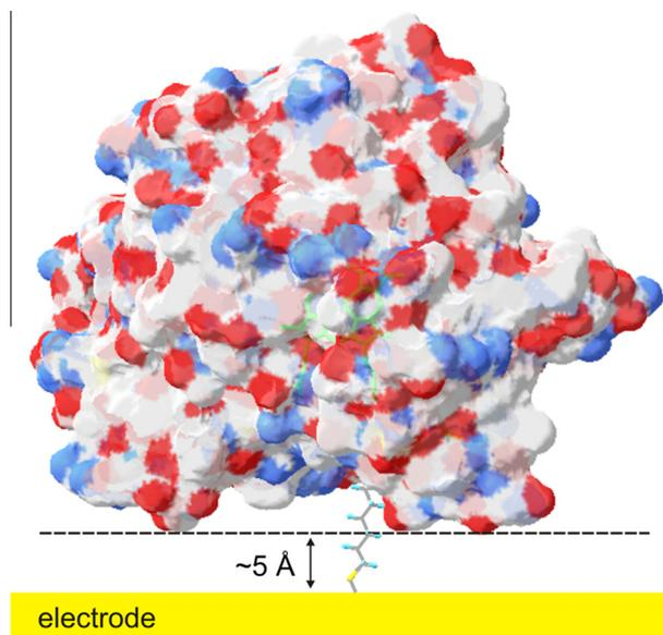
**Fig. 1.** Schematic representation of horseradish peroxidase reconstituted onto hemin covalently attached to 11-aminoundecanethiol linker tethered to the gold electrode and thus correspondingly orientated at the electrode. The HRP molecular structure was from PDB, PDB ID: 1ATJ [51].
