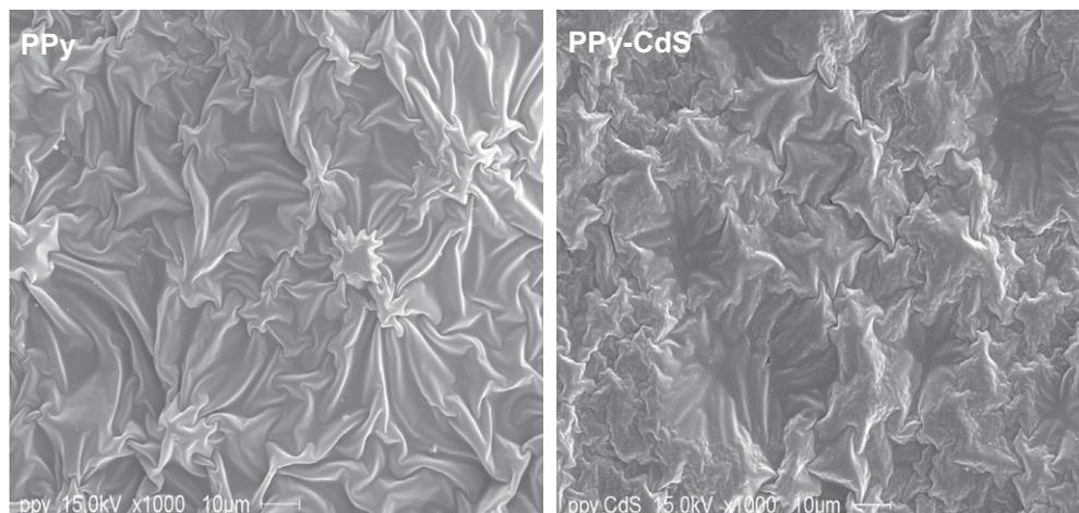
**Fig. 2.** SEM images of PPy and PPy-CdS electrodeposited on ITO-electrode.
