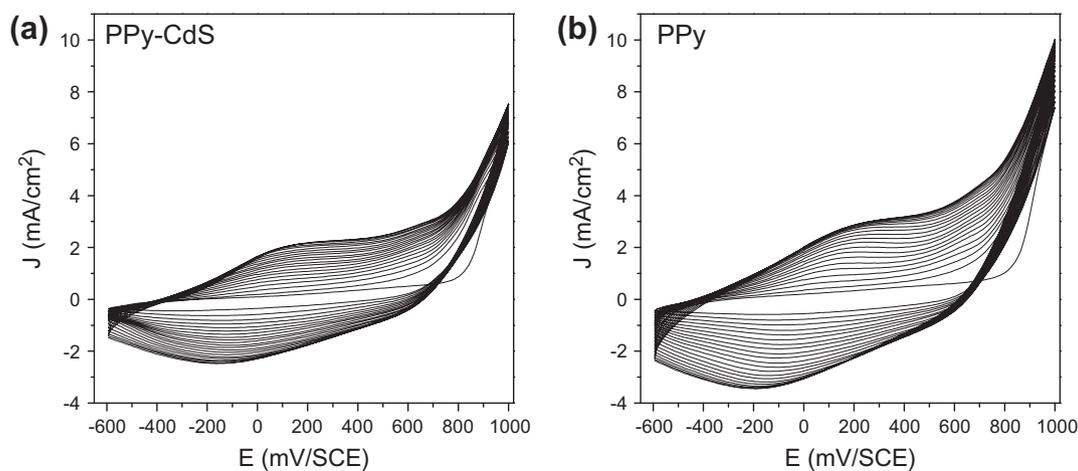
**Fig. 1.** Cyclic voltammograms for the electropolymerization of pyrrole in  $\text{LiClO}_4$  ( $10^{-1}$  M) aqueous solution, in the presence (a) or without (b) CdS ( $10^{-3}$  M). The voltammograms represent 20 sweep segments from  $-0.6$  to  $1.0$  V,  $v = 50$  mV/s.
