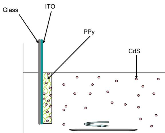
**Scheme 1.** Schematic illustration of preparation of the modified electrode (ITO/PPy-CdS).
