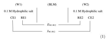
A hydrophilic salt such as KF, KCl, KBr, KI and KClO<sub>4</sub> was used as the supporting electrolyte in the aqueous phases.
