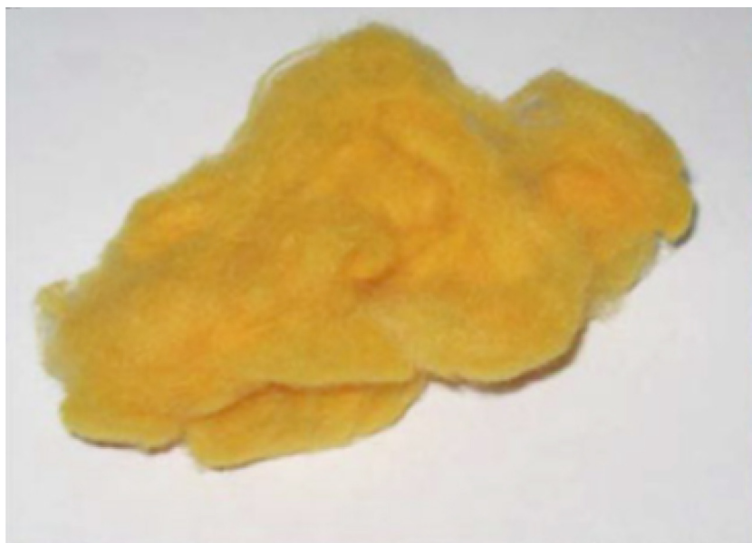
Fig. 1. Ion exchange fibres (IEFs) in staple form [11].
