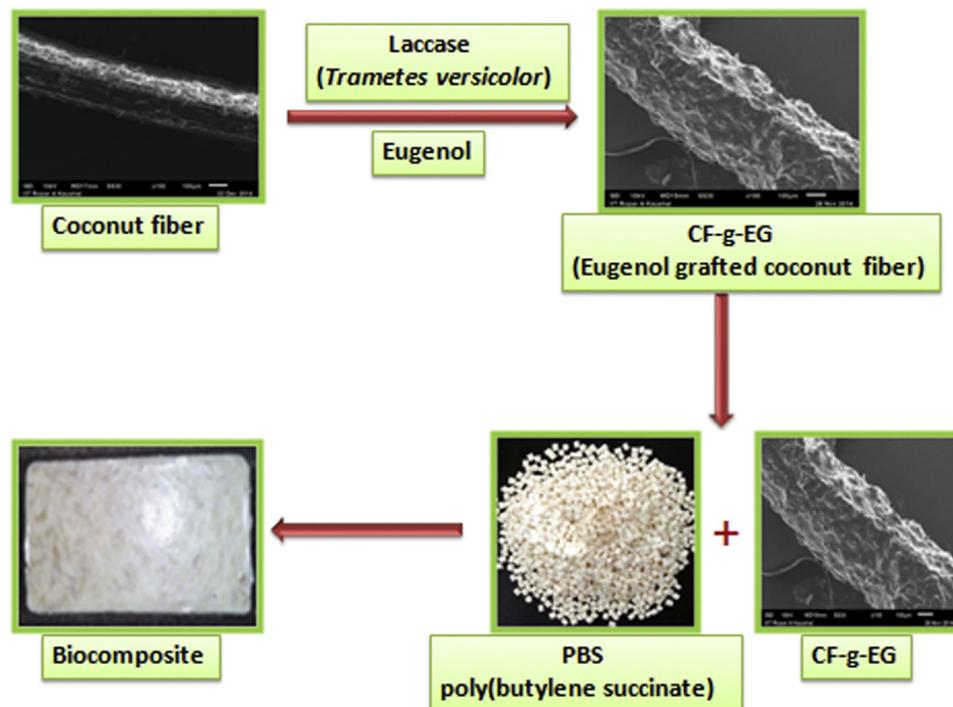
Fig 1. Schematic representation of preparation of biocomposites reinforced with biografted fibers.
