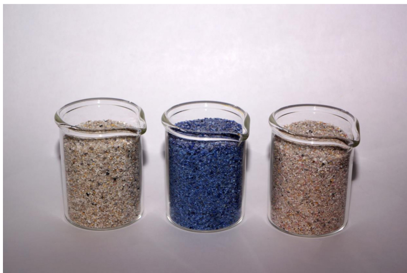
Fig. 1. Photographs of sand from column experiments fed by the three dyes (at 31.5 \mu\text{M} ) for three months: (left) orange II, (middle) methylene blue (MB) and (right) reactive red 120. It is noticeable that sand affinity for MB is high.
