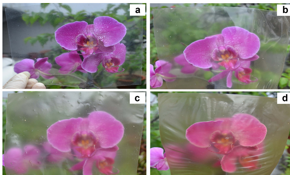
Fig. 1. Flowers wrapped with films of cellulose/STLP composite films with different STLP contents: (a) 0 wt.%, (b) 5 wt.%, (c) 15 wt.% and (d) 25 wt.%.
