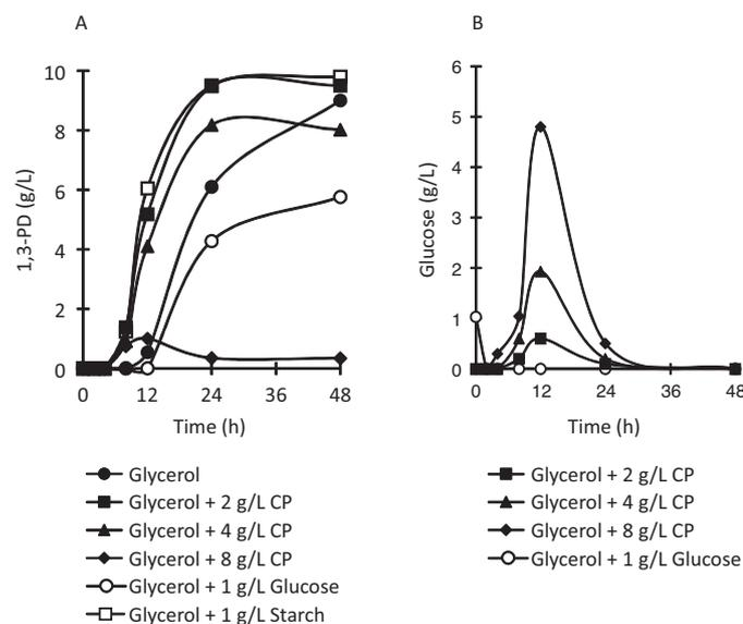
**Fig. 1.** Profiles of fermentative 1,3-PD production (A) and released glucose from CP (B) by *C. butyricum* 15–42 during batch fermentation on M1 medium (containing 30 g/L glycerol) supplemented with CP at various concentrations.
