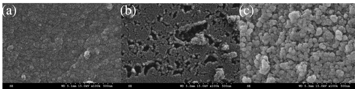
Fig. 2. SEM images of (a) NAC (b) AAC-0.1 and (g) BAC-1 prepared by chemical treatments.
